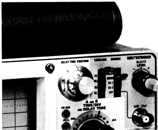
Fig. 1. The TEKTRONIX 475 provides analog sweep delay using a calibrated ten-turn potentiometer. On some scopes this control is called the DELAY TIME MULTIPLIER. The number of dial divisions between the start and the end of delay is multiplied by the TIME/DIV setting, to compute delay.
