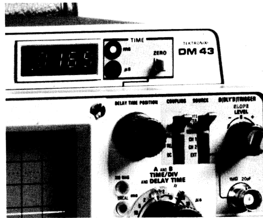
Fig. 2. The TEKTRONIX 475 with DM40 or DM43 provides analog sweep delay with LED readout. The readout is set to zero at start of the delay and the readout shows the delay time when the DELAY TIME POSITION control is set to the end of delay. No calculations are necessary.
